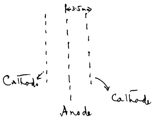
Anode to Cathode Distance  $\approx 3.5 \text{ mm}$
