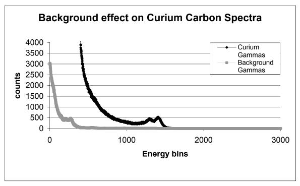
Therefore, we concluded that neutron interactions not simulated by GEANT were probably the cause of most of the observed low energy gammas.
