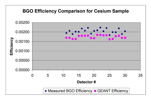
It is apparent that the measured data points all lie above those produced by GEANT and it almost seems as though some sort of linear scaling factor should be added to GEANT points. My thoughts were that this was due to some background effect or an effect of the beta particle, which
