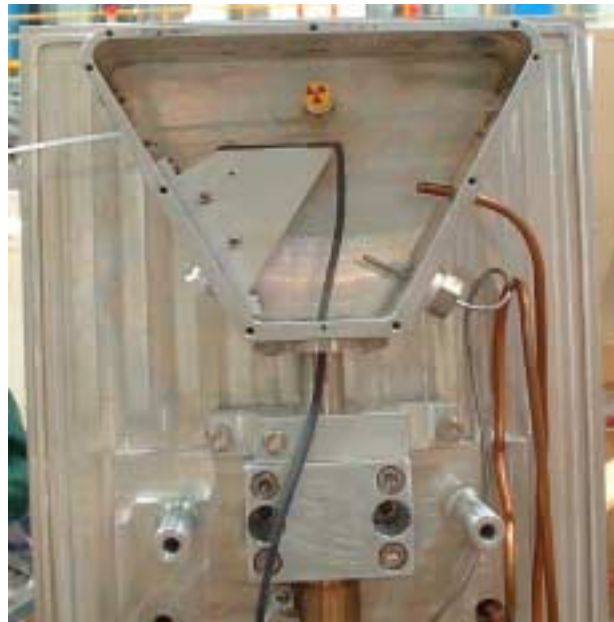
(c) Photo of the gas target showing the ^{244}\text{Cm}^{13}\text{C} source positioned inside
