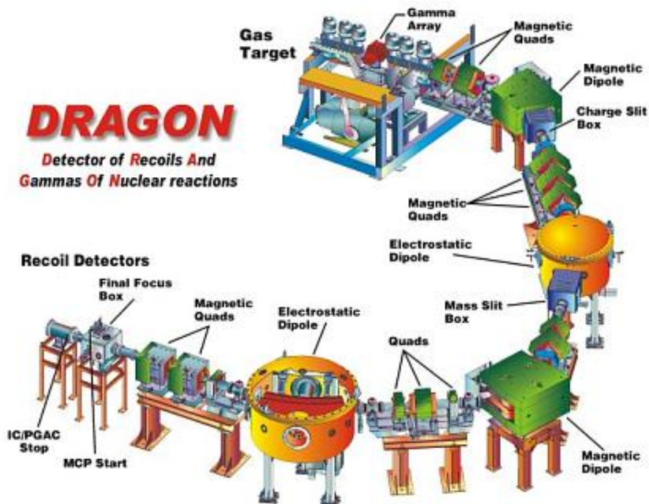
FIG. 1: Schematic overview of the DRAGON apparatus
