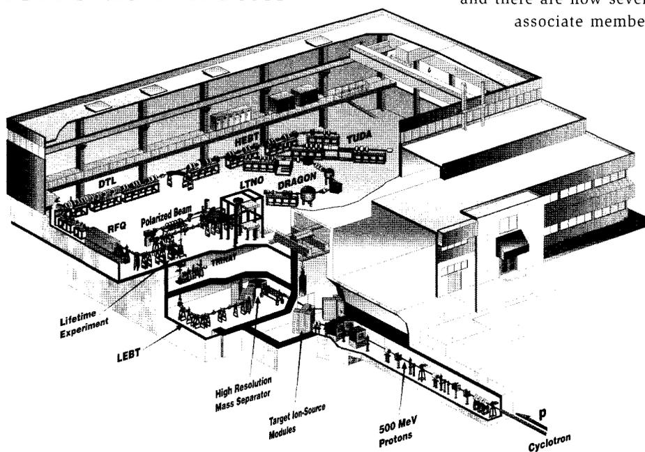
Figure 1. Illustration of the ISAC-I facility at TRIUMF. The 500 MeV protons from the cyclotron strike a thick target producing the radioisotopes. Extraction with the ion source and mass analysis through the separator allow radioisotopic beams to be delivered to any of the experimental facilities. The RFQ and DTL accelerators allow beams to be accelerated up to 1.8 MeV/u.
