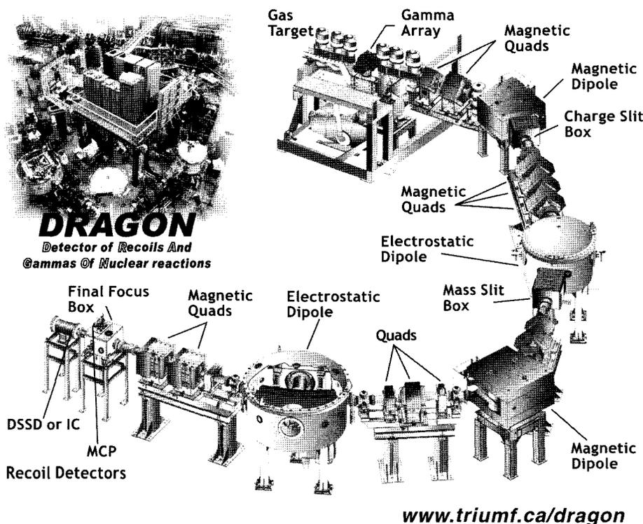
Figure 2. Illustration of the main components of the DRAGON recoil mass spectrometer; the inset shows a photo of the actual device. The unique DRAGON facility allows the measurement of reaction strengths important to understanding elemental synthesis in the universe. DRAGON filters out the interesting product nuclei from these weak reactions with suppression factors of  $10^9$  to  $10^{13}$  possible, depending on the detector configuration and the specific reaction under study.
